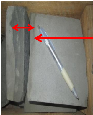
Plate 6.4 Core#1 showing some sedimentary features in well E-A01 displayed in boxes for observation and description (courtesy of PASA).
