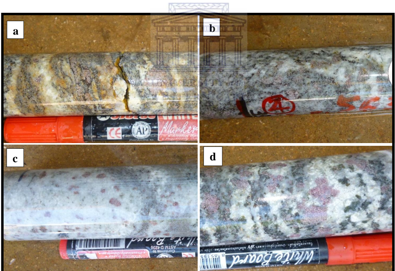
Plate 4-7: : Core photographs showing different variations of the feldspathic biotite garnet gneiss. Variety 1 (a), variety 2 (b), variety 3 (c), variety 4 (d).
