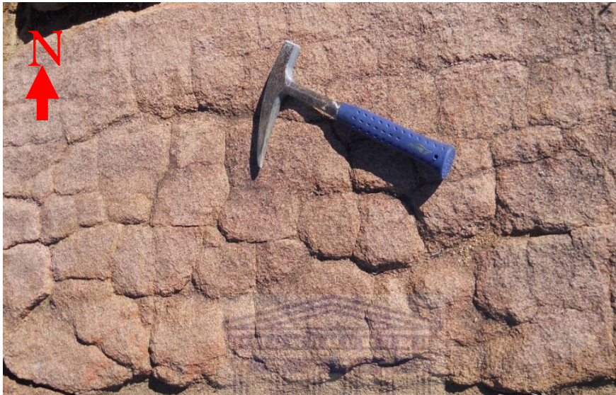
Plate 8-1: Field evidence of “east-west and north-south-south Syn-kinematic joints on the augen gneiss of the Little namaland Siute within the western lense of the Hondekloof deposit.
