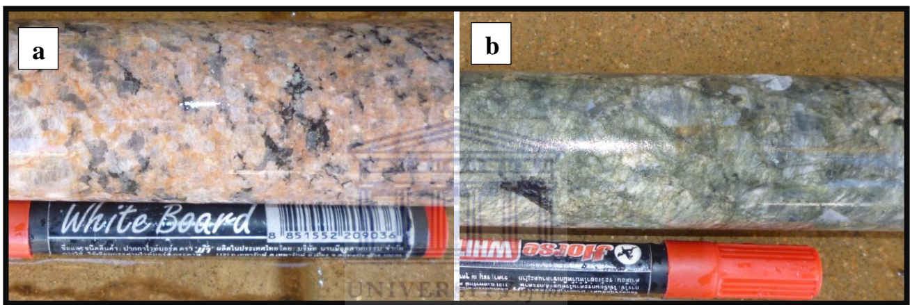
Plate 4-11: Core photographs showing the meta-syenite of the Hondekloof deposit. a. variety 1; b. variety 2.
