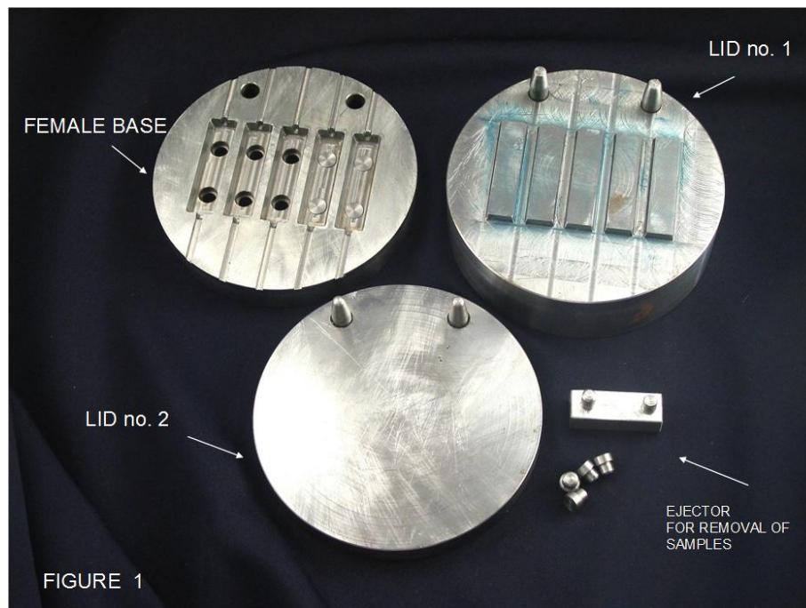
Figure 2.1: Custom made steel template.
