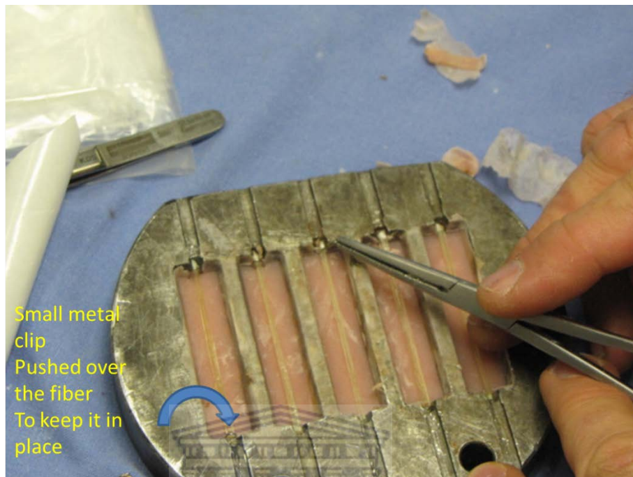
Figure 2.3: "Stapling" the shorter fibres into position.
