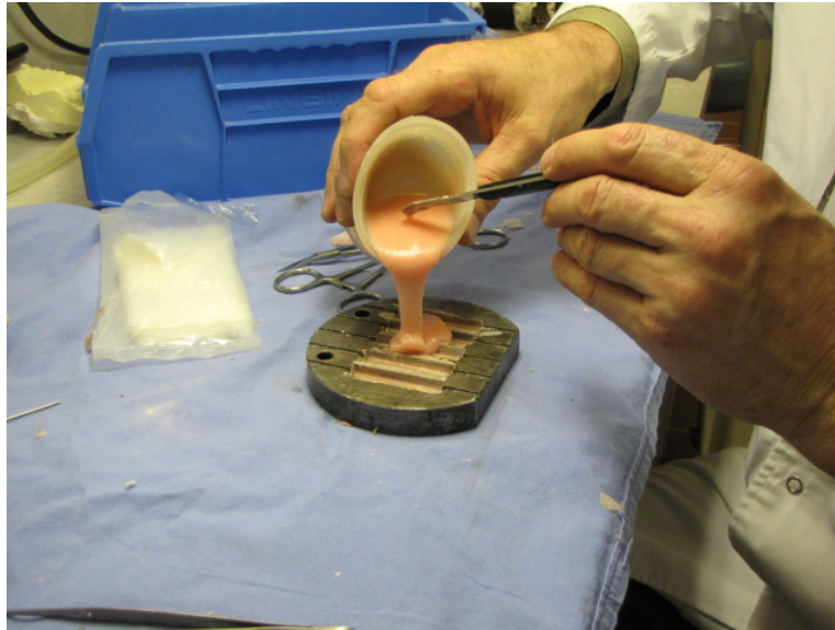
Figure 2.8: The second mixture is placed over the fibres to completely fill the cavities.
