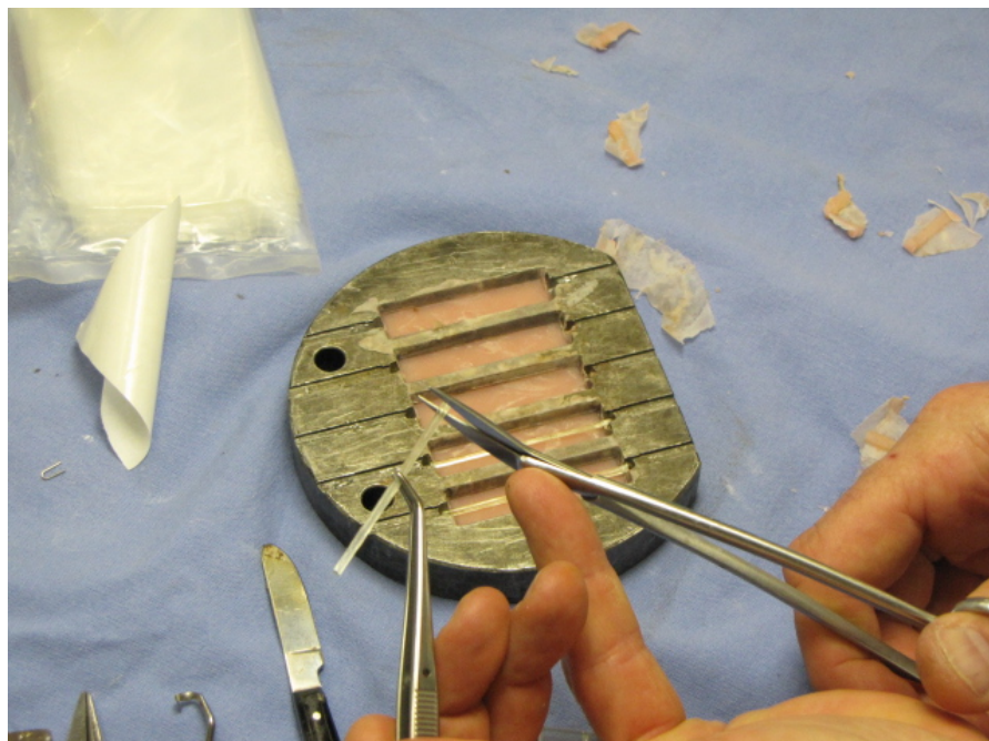
Figure 2.4: Cutting longer fibres to the correct length.
