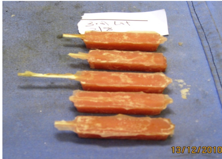
Figure 2.5: Fibres moving during the manufacturing process
