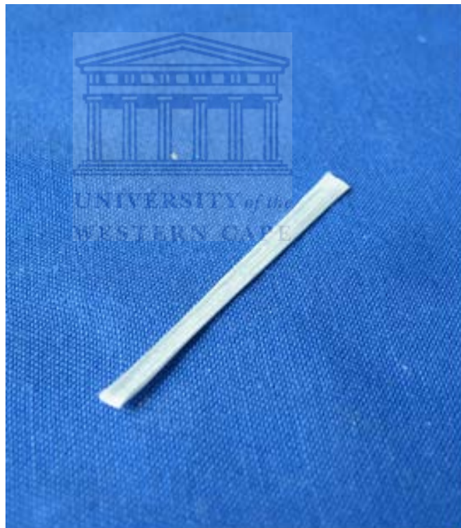
Figure 2.14: Unidirectional, un-impregnated “Stick” fibre
