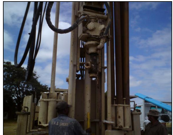
f) Rod end which holds the drill bit
