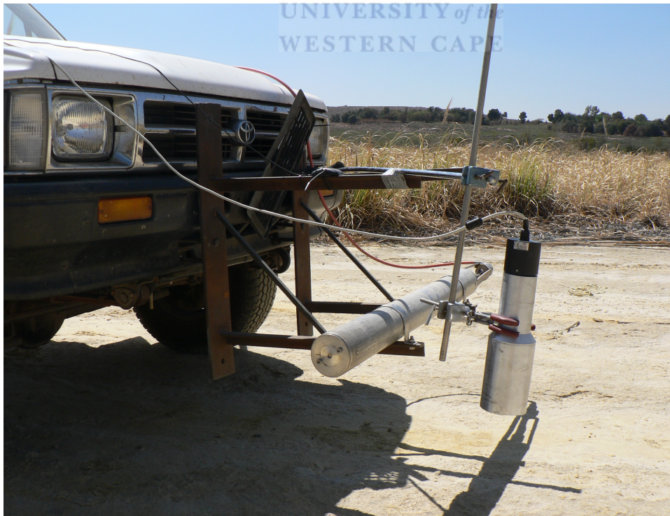
Figure 3.6 The NaI (Tl) detector mounted next to the Medusa detector in front of 4 X 4 vehicle.
