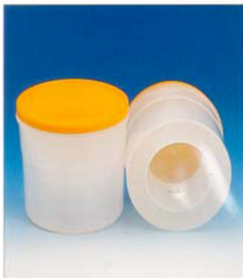
Figure 3.4: Picture of the one litre polypropylene Marinelli beaker (model VZ-1525) used to hold samples for radiometric measurements.
