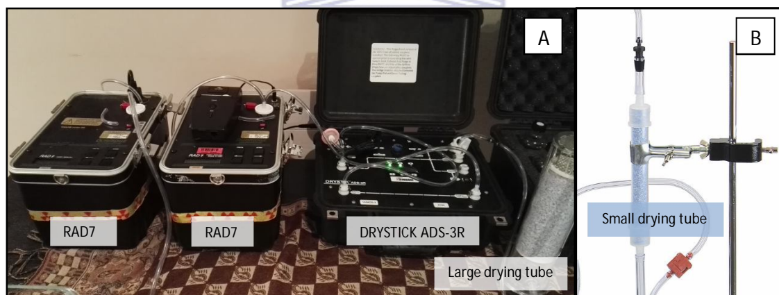
Figure 3-6: DURRIDGE manufactured components to reduce RAD7/s relative humidity (RH): DRYSTICK ADS-3R (A), large laboratory desiccant drying tube (A) and small desiccant drying tube (B).
