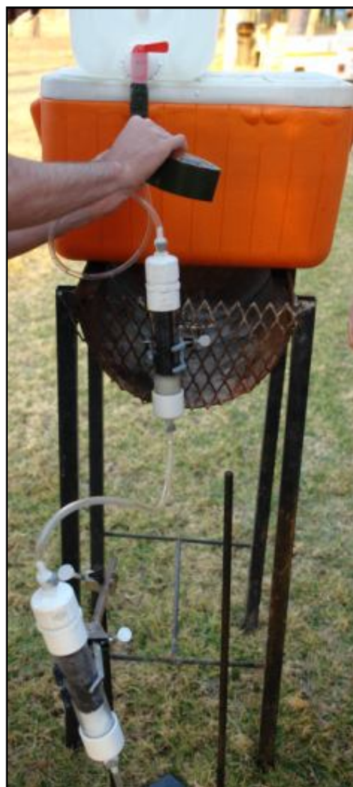
Figure 3-15: Radium isotopes filtering device making use of a gravity feed system and Mn-oxide coated fibbers.
