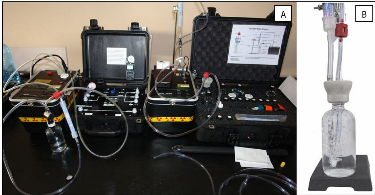
Figure 3-10: Experimental setup (A) to conduct the radon-in-water activity concentration measurements as illustrated in figure 3-9. Aeration process (B) in progress to extract the radon from the water to the air (carrier medium) for a 250 mL vial (RAD H2O, 2016).
