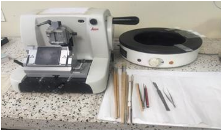
Figure 6: Photograph showing a rotary microtome and a water bath.
