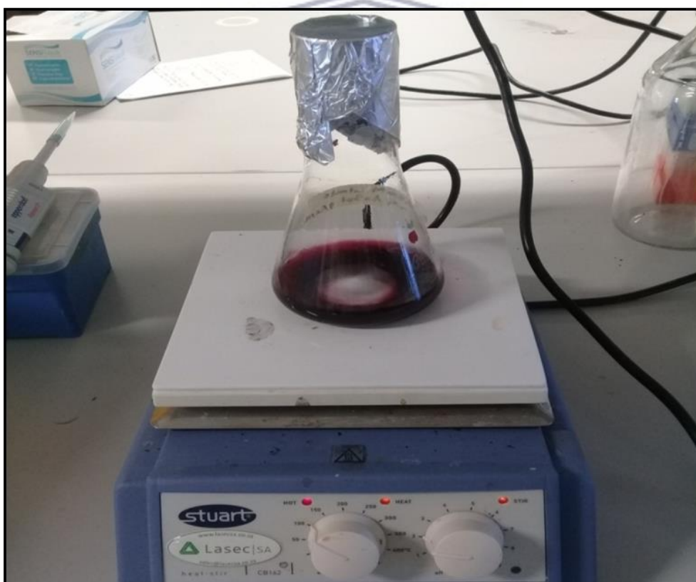
Figure 4.2: General setup for the citrate reduction synthesis of spherical AuNPs at 100 °C.
