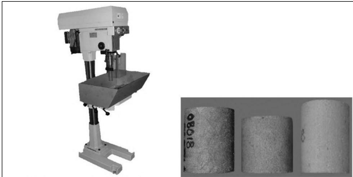
Fig.3.13. Core plug drilling press and typical core plugs (McPhee et al., 2015).
