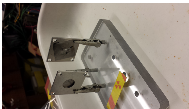
Figure 4.1 – Far target(top) being removed after irradiation and blank target(bottom) before irradiation.
