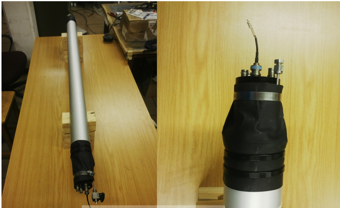
FIGURE 3.9: A photographic picture of the liquid scintillator detector setup.
