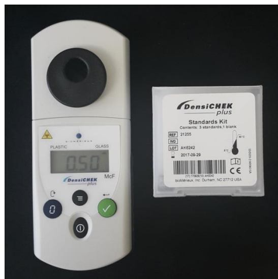
Figure 3-3: DensiCHEK Plus BioMerieux, Inc Durham, USA showing the concentration of the microbial suspension of 0.5 McFarland standard.
