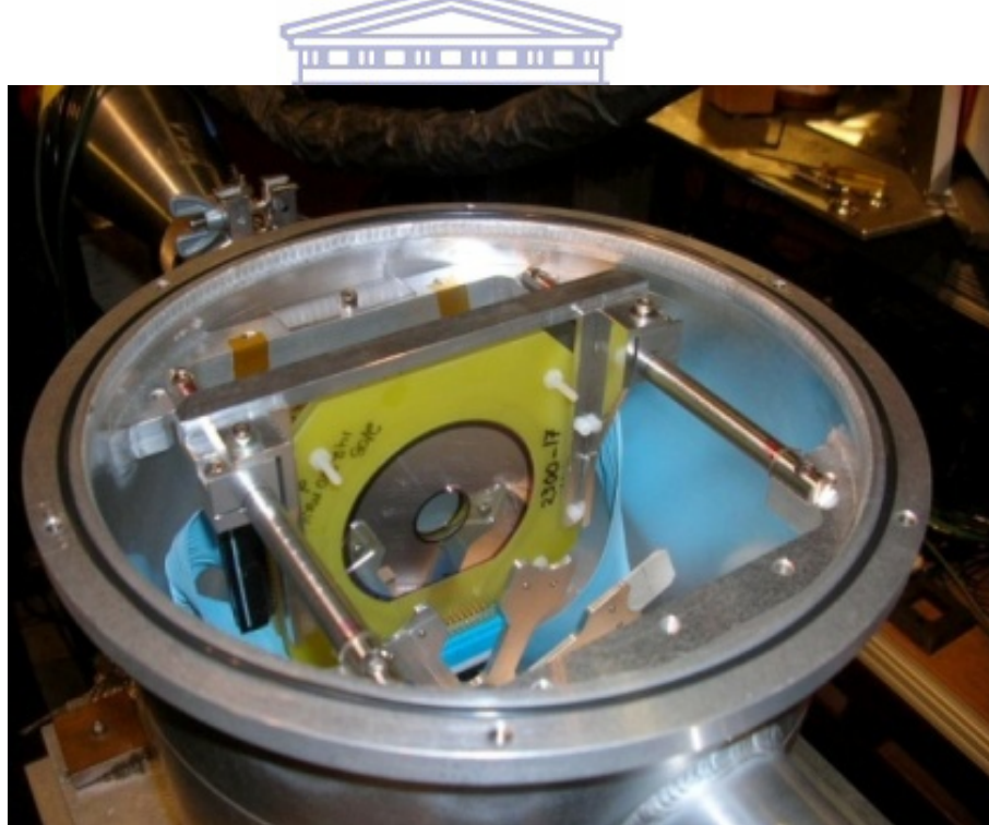
FIGURE 3.3: The Silicon Detector Telescope (SDT) used for proton detection [24].
