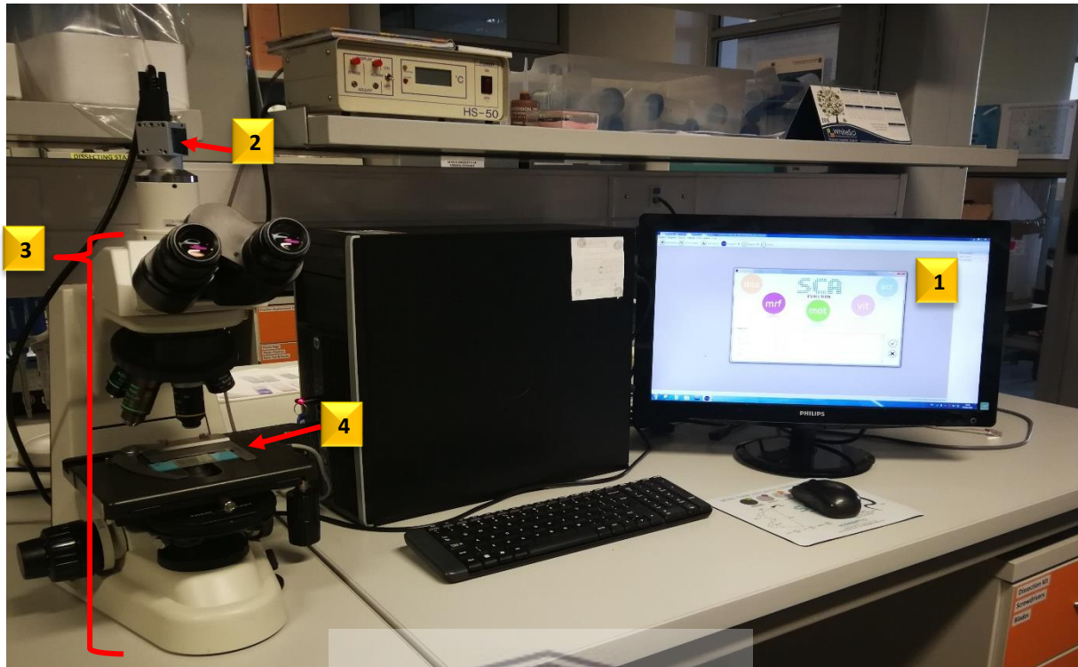
Figure 3.3 Equipment used for the analysis of semen parameters by CASA. 1) Computer with SCA ® software for CASA analysis, 2) Digital camera (Basler ace acA 1300-200uc colour USB 3.0), 3) Nikon Eclipse 50i microscope, 4) Heated stage
