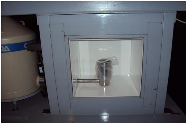
Figure 3.2: BEGe detector in a lead castle.
