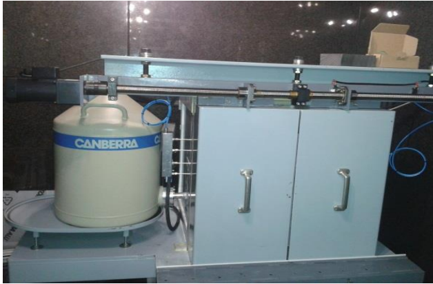
Figure 3.1: Lead castle with sliding doors.
