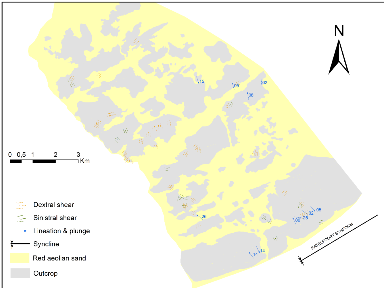
Fig. 4.23. Locations of lineations and shear zones in the Gladkop Suite, south of Steinkopf (this study). The S-shaped symbols are oriented to indicate the linear trend of shear zones. Map symbols are in line with the Federal Geographic Data Committee (FGDC) Digital Cartographic Standard for Geologic Map Symbolization.
