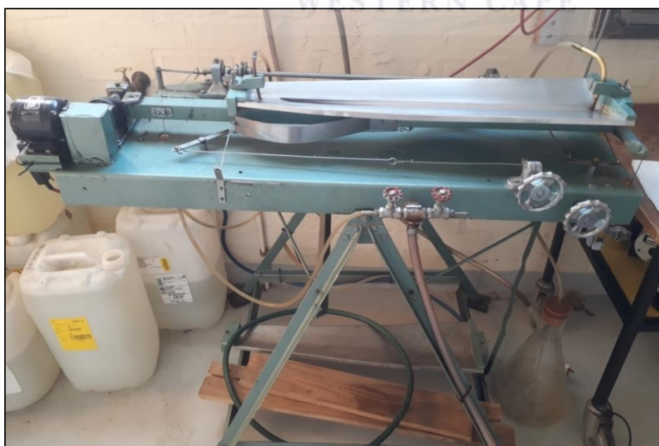
Fig. O.1. Super-panner, which was used for heavy mineral separation of zircon grains, housed at the Central Analytical Facility (CAF), Stellenbosch University.
