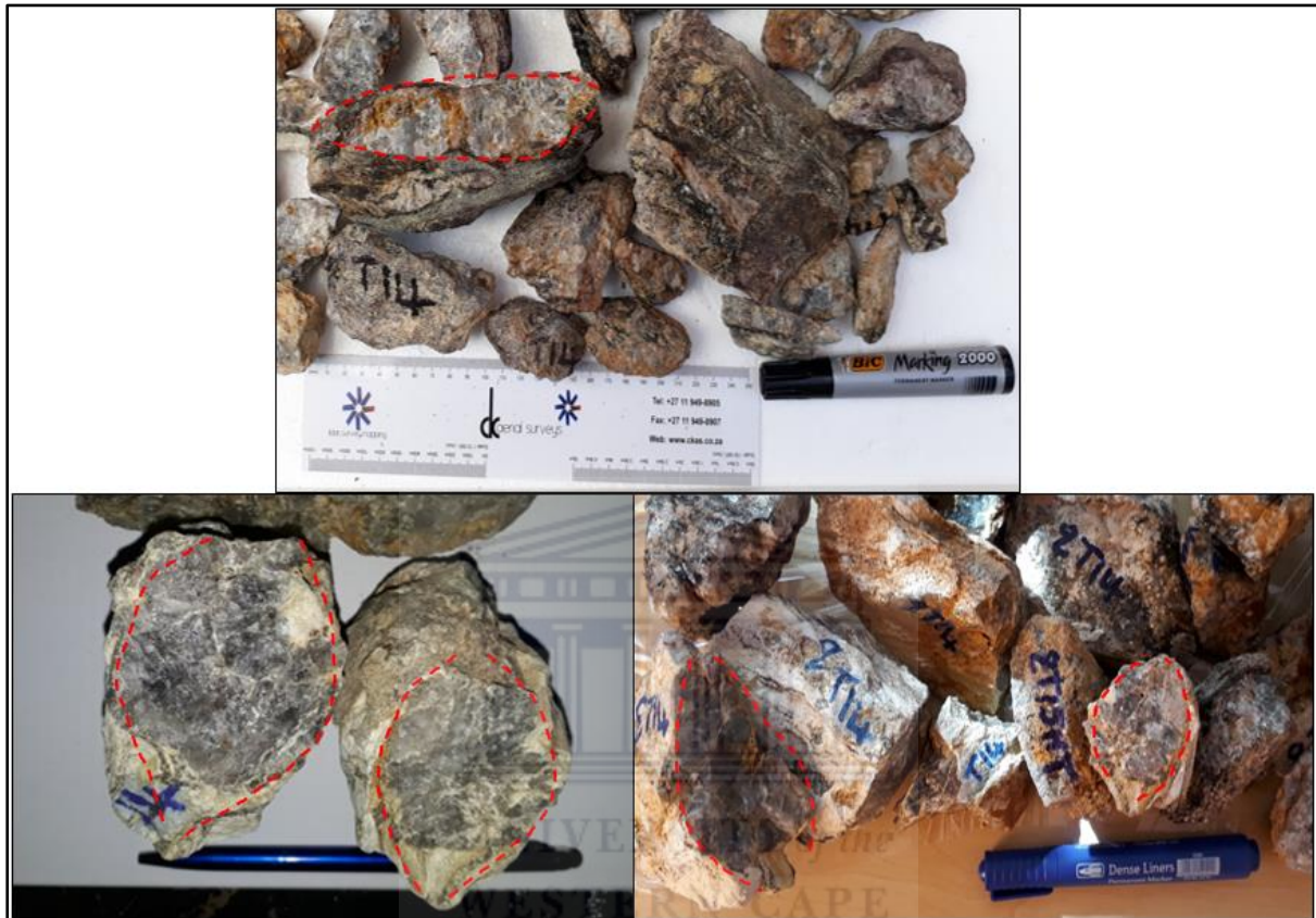
Fig.2.31. Lenticular shaped vein quartz samples from trench 14 (Sandamap), found lying subparallel to the shear-zone schistosity.
