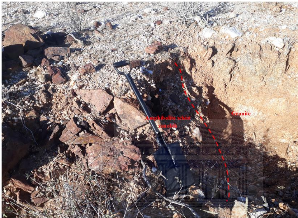
Fig. 2.13. Ferruginous amphibole schist xenolith within the pegmatitic granite in trench 9. The xenolith is partially covered by loose rock debris and some parts can be seen through the rock debris.
