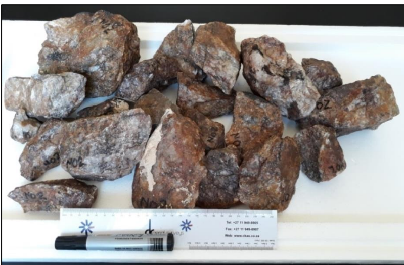
Fig. 2.18. Ferruginous vein quartz samples from a quartz vein in a sheared schist outcrop at sampling point NO2.
