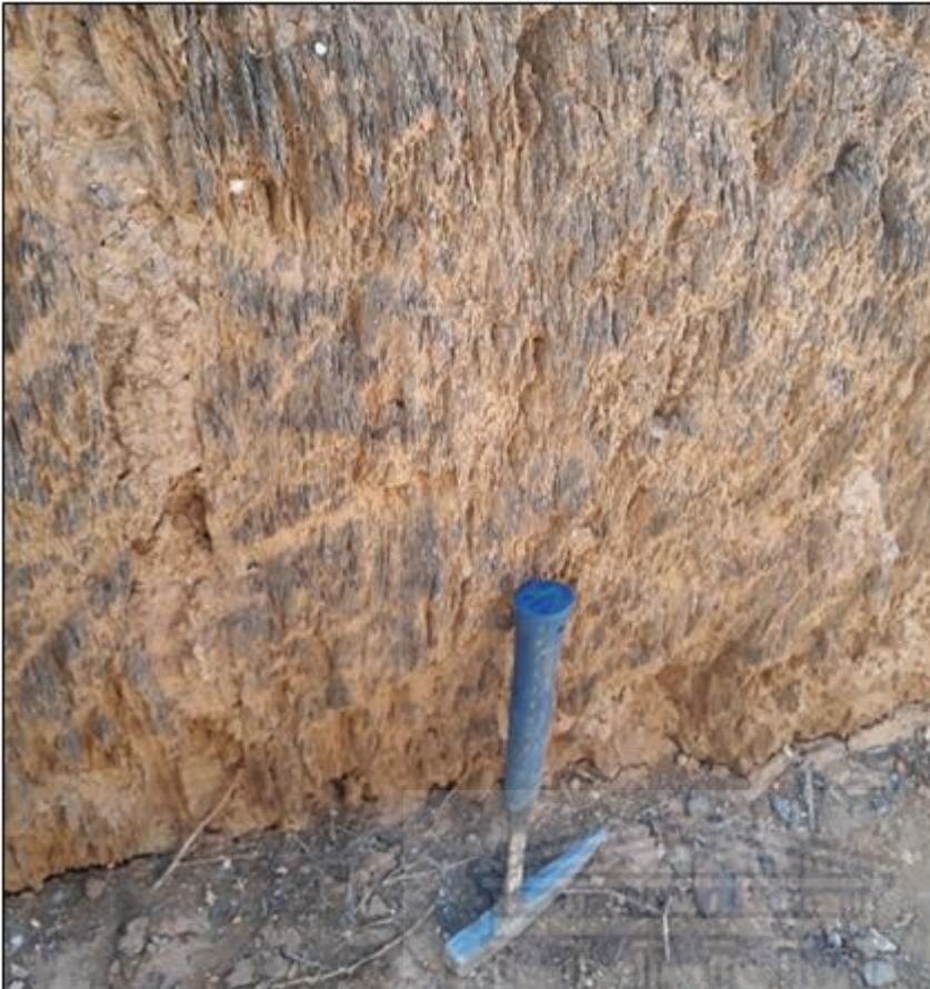
Fig. 2.10. The shear dip is quite steep in some places and in this trench (trench 14) two different measurements were obtained: 70° ESE and 80° ESE.
