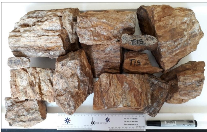
Fig. 2.16. Hydrothermally altered schist samples from trench 15 (T15) which, according to XRD results, are composed of quartz, cummingtonite, calcite, albite, muscovite, mimetite, kaolinite, alunite and dickite.
