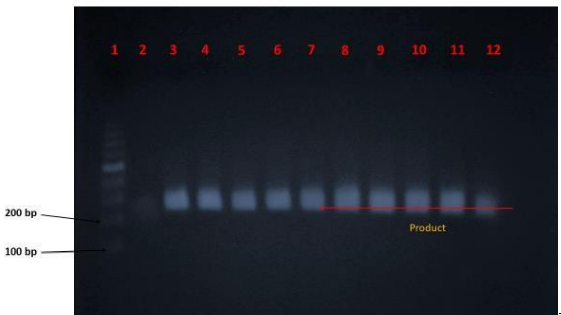
Figure 3.23: Agarose gel electrophoresis of the PEG 10 gene, showing bands of the intended product. Red arrow indicates the product size (253 bp). The gel represented as line 1: 100pb Marker, line 2: N.C (Nuclease-free water), line 3: untreated LNCaP, line 4: treated at IC 25 for 24h LNCaP, line 5: treated at IC 75 for 24h LNCaP, line 6: treated at IC 25 for 72h LNCaP, line 7: treated at IC 75 for 72h LNCaP, line 8: untreated PWR-1E, line 9: treated at IC 25 for 24h PWR-1E, line 10: treated at IC 75 for 24h PWR-1E, line 11: treated at IC 25 for 72h PWR-1E, line 12: treated at IC 75 for 72h PWR-1E.
