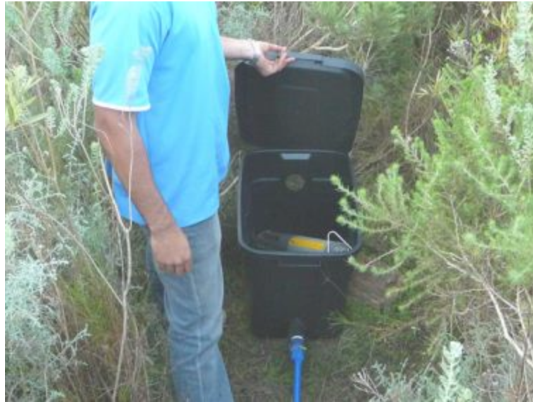
Figure 4.1: Flow cell with the YSI 6600 multi parameter sonde inside it.
