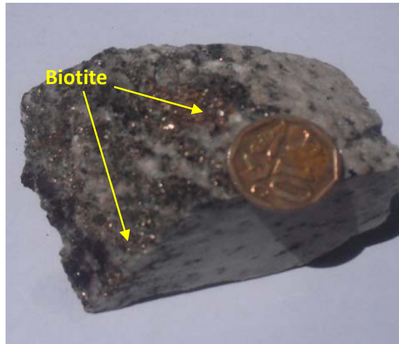
Figure 3.11: Sample of biotite gneiss showing biotite-rich patches. Scale is given by a coin of 1.7 cm diameter.
