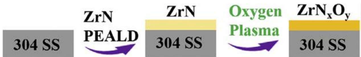
Figure 2.14: Schematic representation for deposition process of ZrN x O y coating on 304 SS [78].
