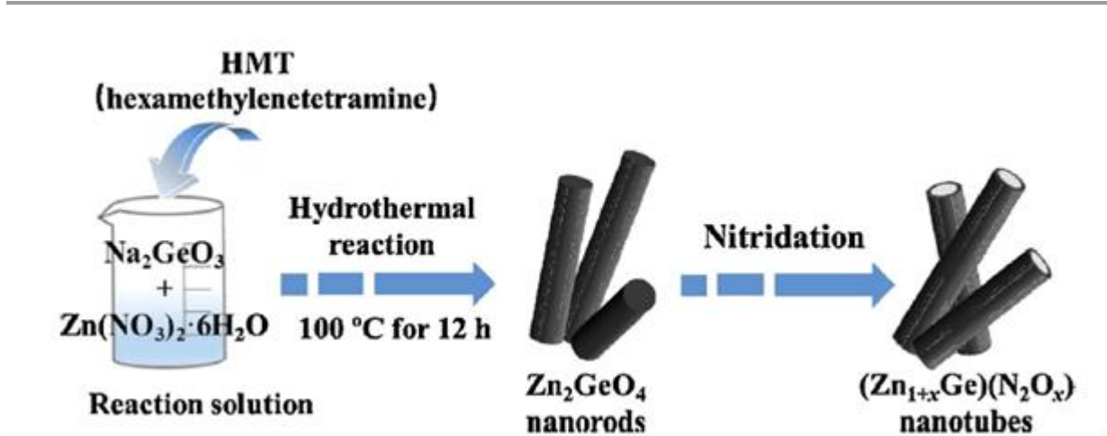
Figure 2.18: Schematic representation for the two-steps preparation process of (\text{Zn}_{1+x}\text{Ge})(\text{N}_2\text{O}_x) nanotubes [97].
