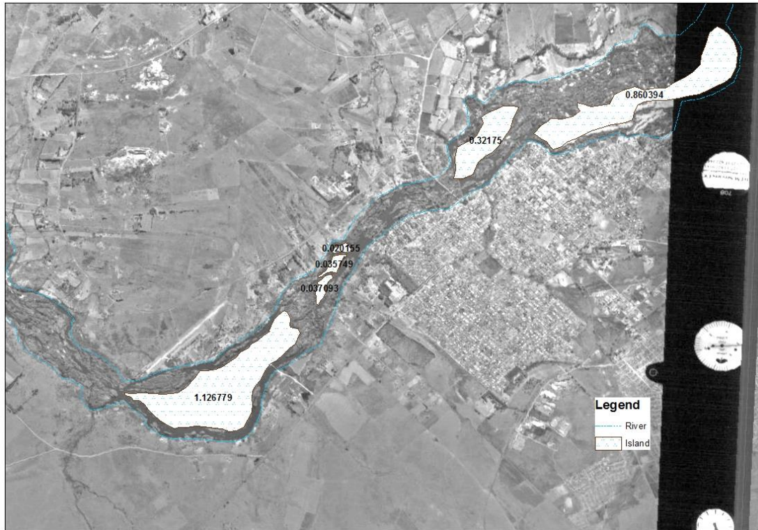
Figure 4. 21: digitized aerial photographs for the year 1991 and 2001, the numbers inside the island represent the area of the island in km 2 .
