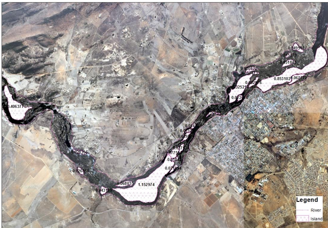
Figure 4. 27: digitized aerial photographs for the year 2012 and 2015, the numbers inside the island represent the area of the island in km 2 .
