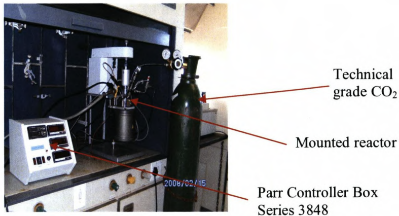
Figure 3.4: The autoclave reactor used in the study and the assembly consisting of the controller, mount and gas cylinder (manufactured by Parr Instruments).
