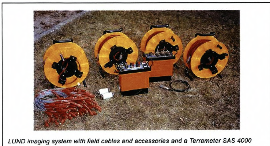
Figure 3.2: Field cables, switching units and a terrameter SAS 4000
