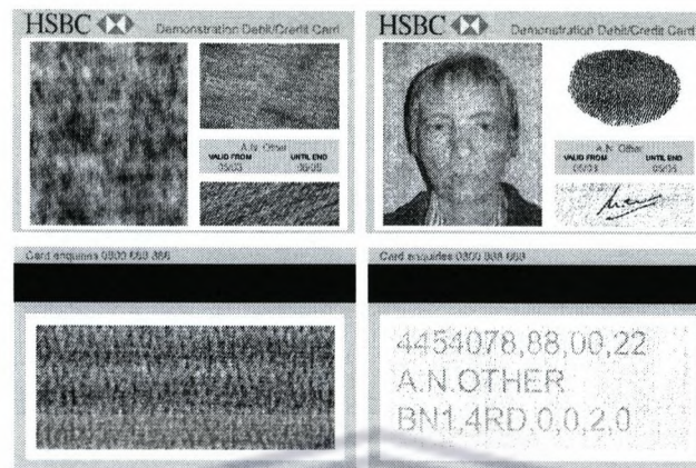
Figure 5.5: Example of the application of ‘diffusion only’ watermarking. In this example, four images of a face, finger-print, signature and text have been diffused using the same cipher and printed on the front (top-left) and back (bottom-left) of an impersonalized identity card using a 600 dpi printer. The reconstructions (top-right and bottom-right, respectively) are obtained using a conventional flat-bed scanner based on a 300 dpi grey-level scan.
