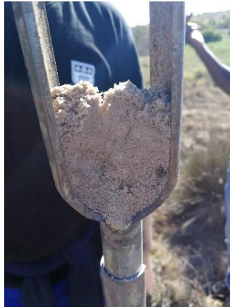
Figure 23: Photo depicting observations of sandy soil sediments via auger investigations at
