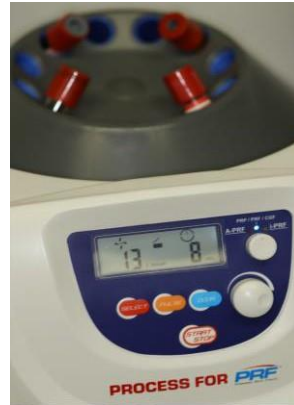
Figure 2: PRF settings and placement of vacutainers
