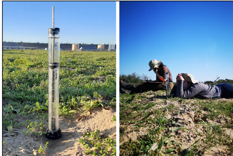
Figure 23: Conducting infiltration tests using the Mini Disc Infiltrrometer
